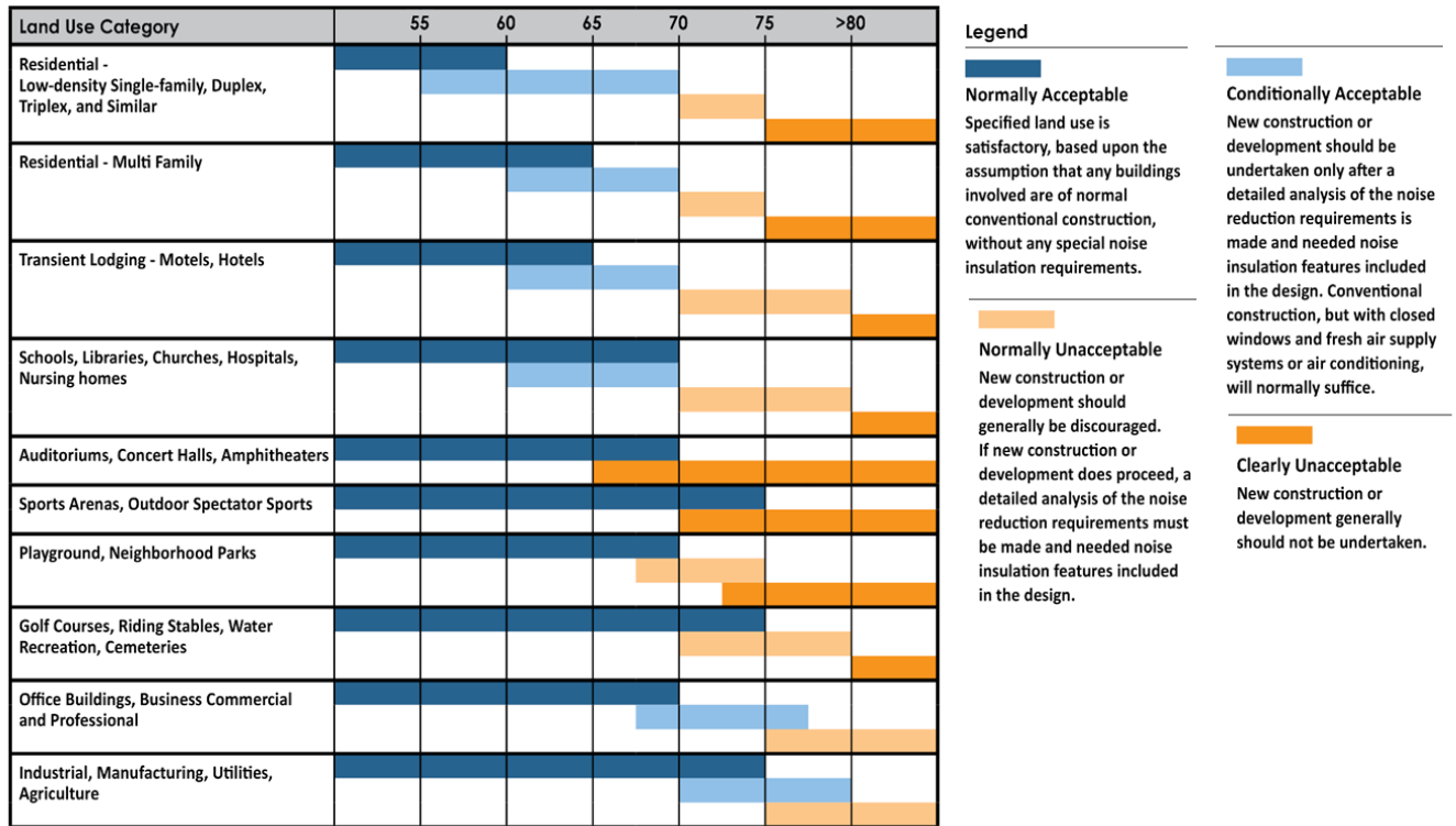
Figure N-2: Community Noise and Land Use Compatibility Guidelines (shown in CNEL, dB)
